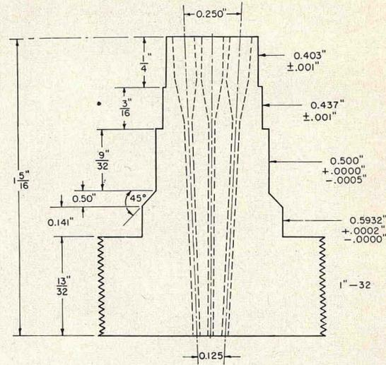
FIG. 7. 7-terminal Be-Cu plug for vessel of Fig. 5. Plug B, Rockwell C 40. The details of the terminals are shown in Fig. 8. A drive plug with a 1 1/4 in.-12 thread backs up Plug B. The extractor and washer assembly are similar to those in Fig. 6.
