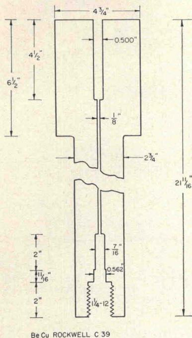
FIG. 4. Be-Cu pressure vessel.
