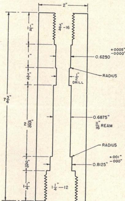
FIG. 11. Be-Cu pressure vessel for microwave measurements.
