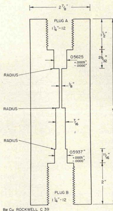
FIG. 5. Be-Cu pressure vessel for work to 20 000 kg/cm<sup>2</sup>. Diameters given are before pressure stretching.
