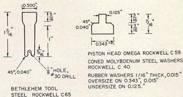
FIG. 3. Piston and packings for liquid tests.
