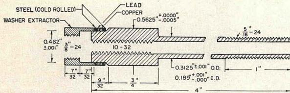
FIG. 6. Sealing plug for Be-Cu vessel of Fig. 5. Plug A. The tubing used in the above plug is 3/16 in. o.d. A drive plug with a 1 1/4 in.-12 thread backs up plug A.
