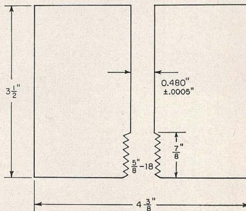
FIG. 14. Stainless steel pressure vessel. Rockwell C 32.
